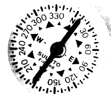
The compass is rotated till the north' marking coincides with the end of the needle pointing north.
